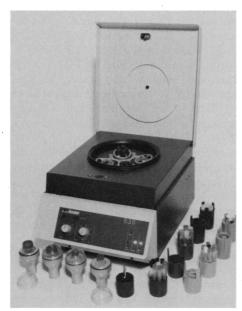
carriers allow 15-ml and 50-ml conical tubes to be centrifuged. Aerosol containment covers are available to safely centrifuge toxic or pathogenic samples. B311 standard features include closed loop speed control, digital speed readout, dynamic electric braking, and imbalance detection and shutdown system. Jouan. Circle 540.
