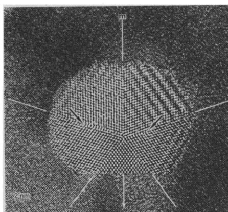
Fig. 1. High-resolution micrograph of a pentagonally twinned germanium precipitate in an aluminum matrix with the beam direction along <110> Ge and <100> Al. The specimen was water-quenched from 450°C and aged for 1 hour at 240°C.
