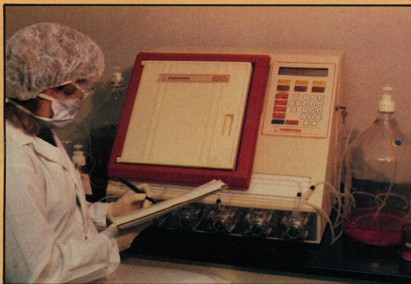
The ACUSYST-Jr.™ cell culture system contains a single bioreactor within the pre-sterilized disposable flowpath with microprocessor control of culture conditions.
