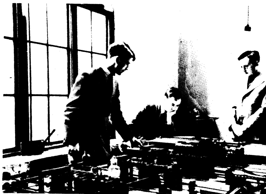
"The model differential analyser in Cambridge." Left to right, A. F. Devonshire, J. Corner "following a curve on the input table," and M. Wilkes. [From Memoirs of a Computer Pioneer ]
