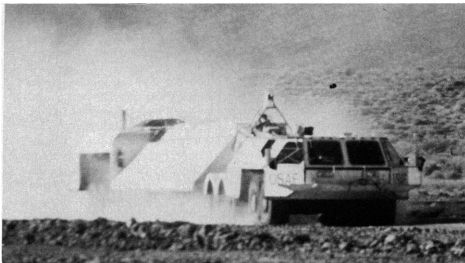
Midgetman launchers. This prototype, constructed by Boeing Aerospace, was designed to move at 30 miles per hour over dirt roads. One of two competing models, it is also hardened to resist overpressures of 30 psi caused by a nuclear blast.
