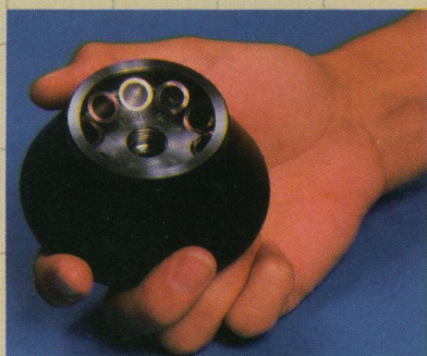
TLA-100.2 Fixed Angle Rotor, 100,000 rpm, 436,000 g
