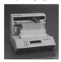
for adaptation to the user's need. Adaptiveslope peak detection assures collection of pure compounds. The stationary rack system accommodates 14 different racks for various sized vessels from 96-well plates to 13 by 100 mm tubes. Removable pans and drain trough simplify cleanup. An optional three-way valve enables the user to divert eluent to the drain. Gilson Medical Electronics. Circle 529.
