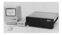
mentation vessels, each vessel would have temperature, pH, agitation speed, and oxygen concentration monitored and maintained. The Proteus unit would provide sensor signal conditioning, set-point control, and communication with a host computer. Each Proteus unit offers display of parameter status and is able to function without the host computer, if necessary. Modular construction provides ease of access and service. Holtz Bio-Engineering. Circle 592.
