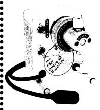
It provides a simple, low-cost means of dispensing very small amounts of fluids for applications such as pipeting, reagent preparation, syringing, precision sampling, repetitive and volumetric dispensing. The variable displacement, valveless RR piston design makes it possible to dispense volumes of 2 to 100 µl per shot with incremental adjustment of less than 0.5 µl. PiP units are also reversible for aspirating fluids or back flushing the system.
