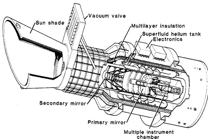
Fig. 6. Cutaway drawing of the SIRTf telescope, showing a number of major subsystems.
