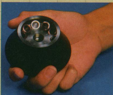
TL-100.2 Fixed Angle Rotor, 100,000 rpm, 436,000 g
