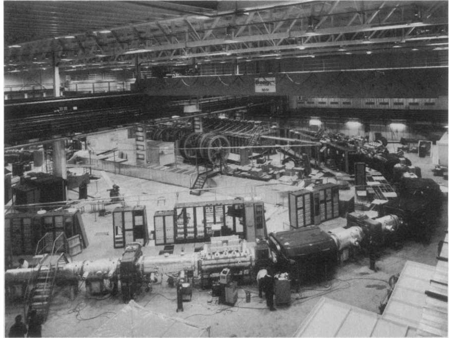
Fig. 12. View of the AA ring before it was covered by concrete slabs. The silvered material around the vacuum tanks is insulation, needed because everything may be heated to 300°C to obtain ultrahigh vacuum. The transmission lines crossing the ring and carrying the cooling signals are also shown.
