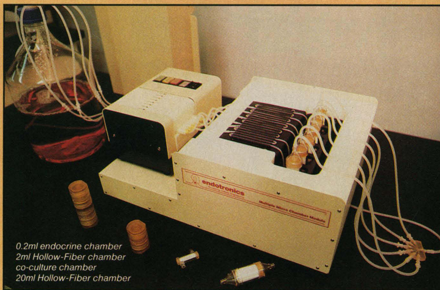
The system can be set-up for recirculation of media to reduce usage when producing antibodies, or connected to a fraction collector to assess endocrine secretions in a time variant manner.
