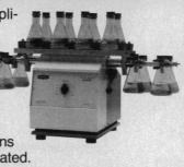
With the Burrell Build-Up® System, capacity can be increased with longer side-arms and platform clamps for various containers. Erlenmeyer and 250 ml flasks or separatory funnels up to 2,000 ml can be easily attached.
