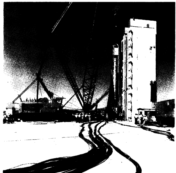
A nuclear bomb is lowered into a hole at the Nevada Test Site. The cables relay detailed information that is then used to modify and improve bomb designs.
