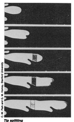
Sequence of growth stages for viscous fingering when the surface tension at the interface between the fluids is low. Times are 90, 110. 140, 171, and 210 seconds after the start of the experiment.
