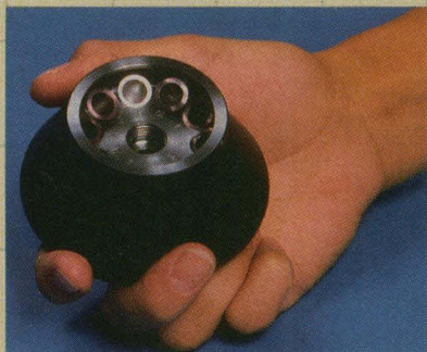
TLA-100.2 Fixed Angle Rotor, 100,000 rpm, 436,000 g
