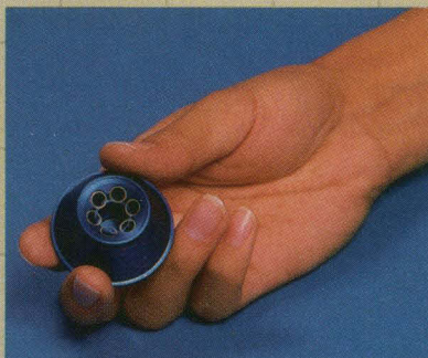
A-100/30 Fixed Angle Rotor, 92,000 rpm, 167,000 g
