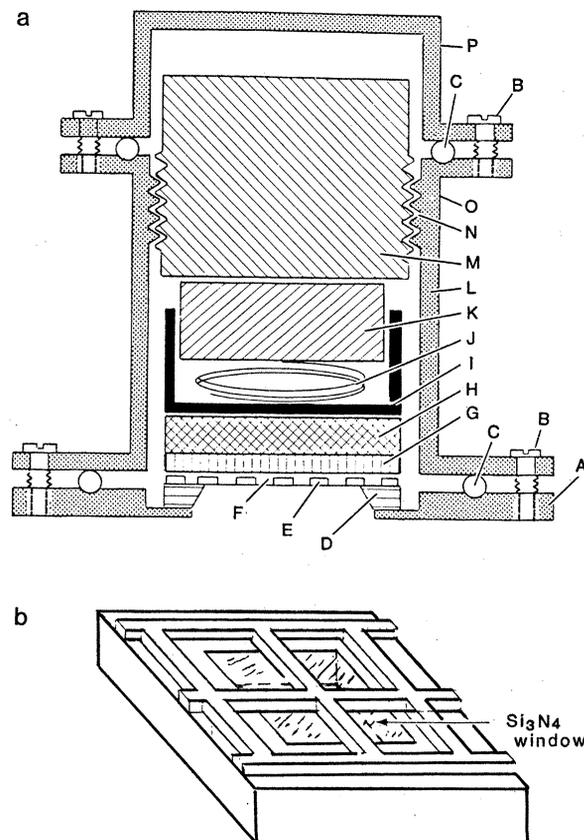
Fig. 1. (a) Diagram of the wet chamber, showing the (A) substrate holder, (D) substrate for vacuum window, (E) resist honeycomb, (F) specimen area, (G) recording resist, (H) substrate for resist, (H to K) spring mechanism to hold resist in position, (B, C, and L) body of wet chamber with O-ring seals, (M and N) threaded spring compressor, and (P) top of chamber. (b) Honeycomb subchamber [enlarged view of (E)].
