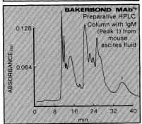
**BAKERBOND MAb** HPLC Columns give a fast, one-step purification of monoclonal antibodies.
