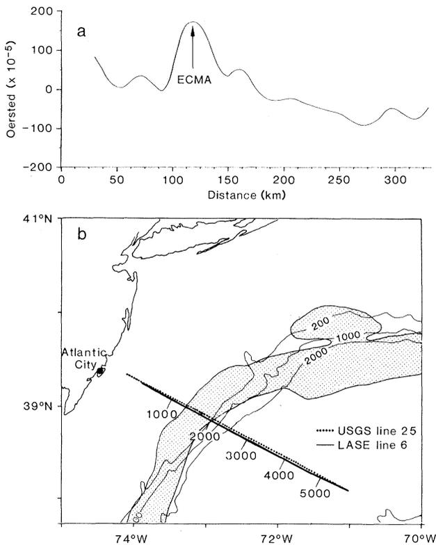
Fig. 2. (a) The magnetic amplitude observed along USGS line 25. The peak of the ECMA is indicated. (b) USGS line 25 and LASE line 6. The stippled area represents the peak of the ECMA. Along USGS line 25, the peak of the ECMA lies entirely on the shelf. Several common-depth-point numbers are indicated on LASE line 6 to facilitate comparison with Fig. 1. Bathymetric contours are in meters.
