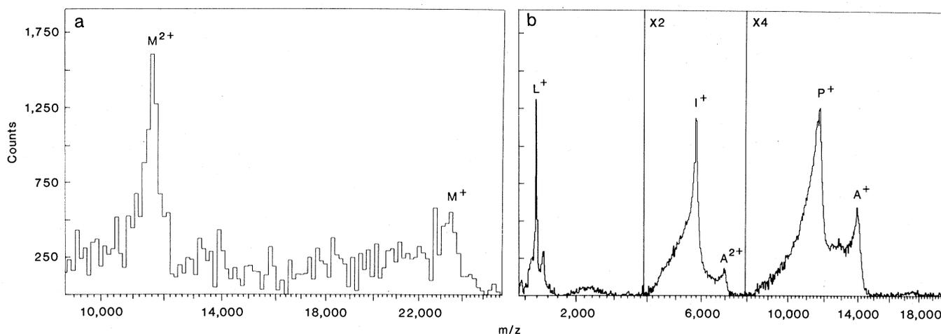
Fig. 1. (a) Positive-ion mass spectrum of porcine trypsin ( $m/z$ , mass-to-charge ratio). The molecular weight determined from the centroids of the  $M^+$  and  $M^{2+}$  peaks is  $23,406 \pm 140$  (calculated MW is 23,463). (b) Positive-ion mass spectrum of a mixture of LHRH (L), porcine insulin (I), pancreatic spasmolytic peptide (P), and phospholipase A2 (A).
