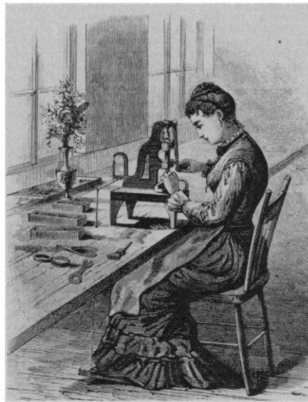
"Punching Out Needle Eyes, Wheeler and Wilson Manufacturing Company, 1879. A series of small, hand-operated machines were used to manufacture sewing machine needles. Two of the most difficult operations included punching out the eye and grooving the needle. The final step of straightening the needles was done by hand with a hammer." [ Scientific American 3 May 1879; Eleutherian Mills Historical Library. From From the American System to Mass Production, 1800–1932 ]
