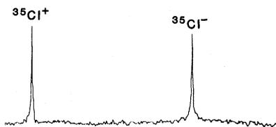
Fig. 1. FT mass spectra of  $^{35}\text{Cl}^+$  and  $^{35}\text{Cl}^-$  at a pressure of  $10^{-8}$  torr and a mass resolution of  $\sim 1,500,000$ . The  $\text{Cl}^+$  and  $\text{Cl}^-$  ion signals were alternately acquired, stored, and transformed. The FT mass spectrometer cannot simultaneously store positive and negative ions. [Reprinted from (11a) with permission]
