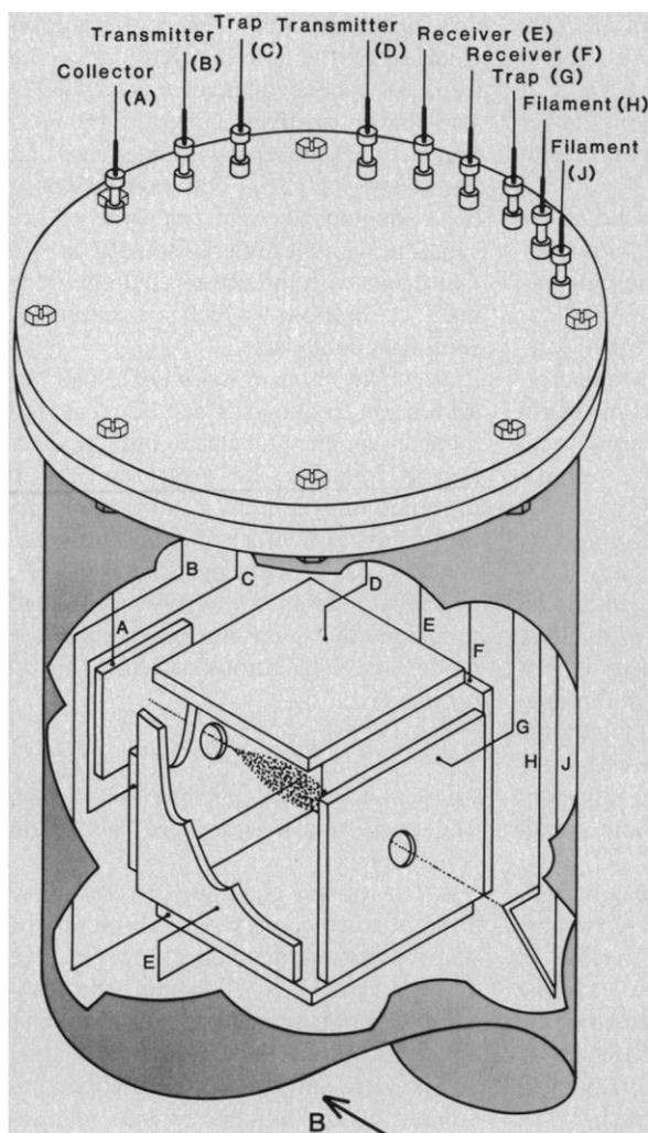
Fig. 2. The cubic ion trap located in a vacuum chamber and between the pole caps of an electromagnet. Ions are formed along the electron beam and probably assume the distribution shown in the cell.
