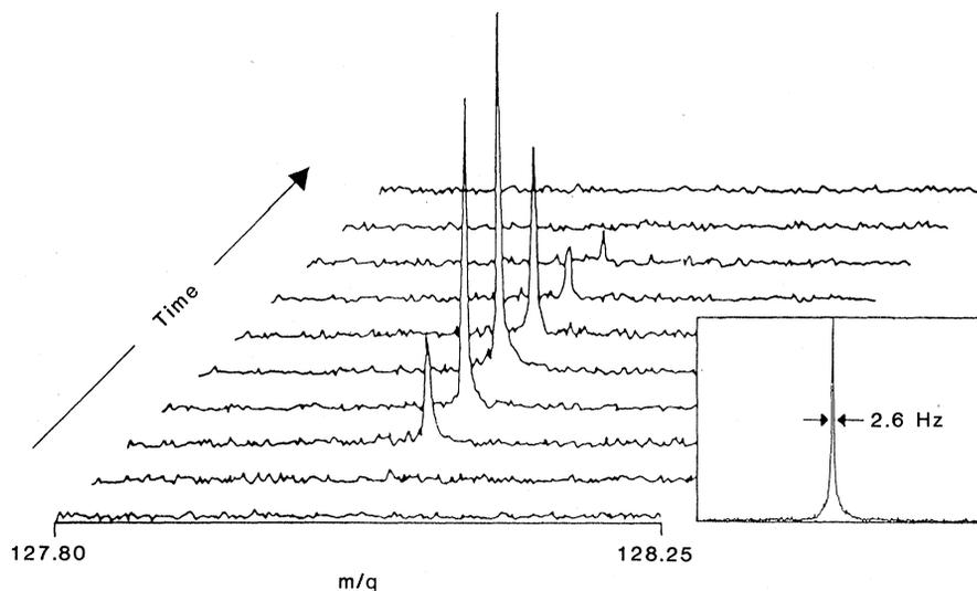
Fig. 3. Elution profile of 20 ng of naphthalene as observed by monitoring the molecular ion at a resolution of 32,000 FWHH. Each spectrum is the result of one 1-second scan. Inset is a higher resolution experiment at 63,000. [Reprinted from (38) with permission. Copyright 1983 American Chemical Society]
