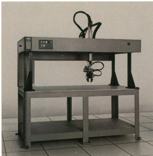
Figure 1. IBM's robotic control language, AML (A Manufacturing Language), is used in all robotic systems that IBM markets. Shown here is the high-end product, the IBM 7565 Manufacturing System, which represents leading-edge technology in intelligent robotics for complex assembly. This system is controlled by an IBM Series/1 computer that monitors manipulator position and sensory feedback 50 times per second, making real-time adjustments if necessary. IBM's mid-range products use AML/Entry, a simplified version of AML, enabling them to be programmed with IBM Personal Computers.
