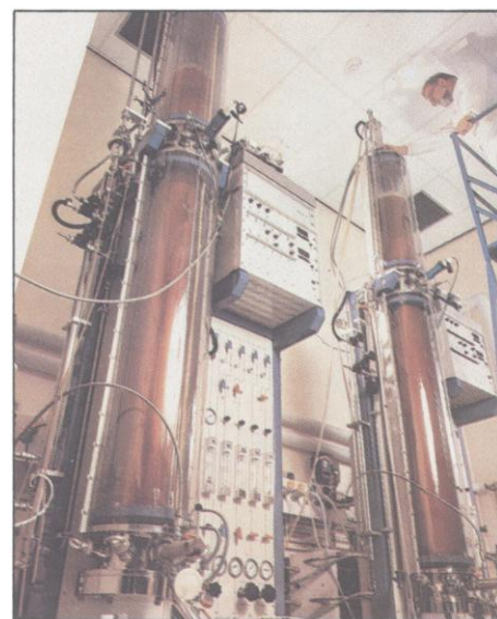
L.H. 2000 Series Fermenters for research use at CAMR, Porton
