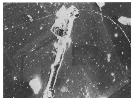
Fig. 4. Secondary electron image stereopair of the furrow. The image on the left is tilted approximately 15^\circ on an axis in the plane of the page. The stereopair shows the topography of the furrow. Scale bar, 40\text{ }\mu\text{m} .
