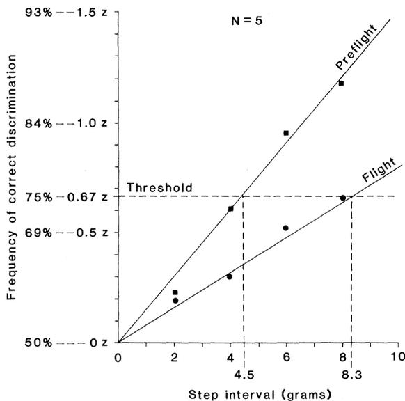
Fig. 1. Mass discrimination under 1 g before flight and under 0 g in flight.
