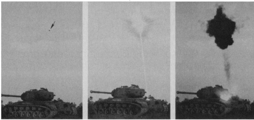
In this 1982 test of Assault Breaker technology, the Avco Corporation launched a submunition from the ground and successfully struck a stationary M60 tank containing a simulated heat source.
