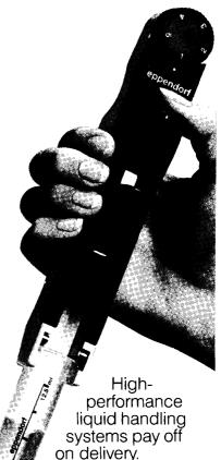
The Repeater dispenses up to 48 samples, without refilling, at 1-second intervals. The six different types of Combitip™ give you a choice of 22 different volumes, from 10 µL to 5 mL, and a large volume selection dial gives you a choice of five different volumes for each Combitip. The Combitip is disposable but can be re-
