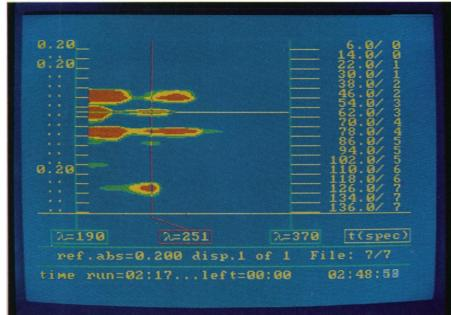
A computer generated contour map of the total absorbance pattern after separation - colour coded to show different levels of absorbance for each isogram. The vertical and horizontal axes are time and wavelength respectively. Built-in cursors let you slice through the isogram in both time and wavelength domains.
