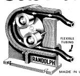
Designed to eliminate all contact of moving parts with the materials being pumped. Ideal for numerous applications where pumping corrosives, abrasive slurries, sterile solutions or gases is a problem. Many models. Capacities from 48 cc to 1,200 gallons per hour.
