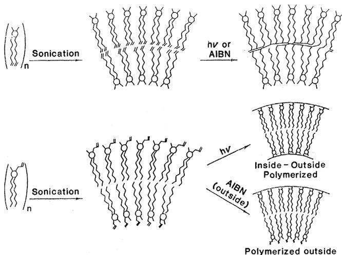
Fig. 1. Schematic representation of vesicle polymerization in the bilayer or at the outer and or inner surfaces.
