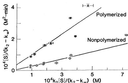
Fig. 6. Kinetic treatment hydrolysis of PNPL in nonpolymerized and polymerized vesicles as given in Eq. 16.
