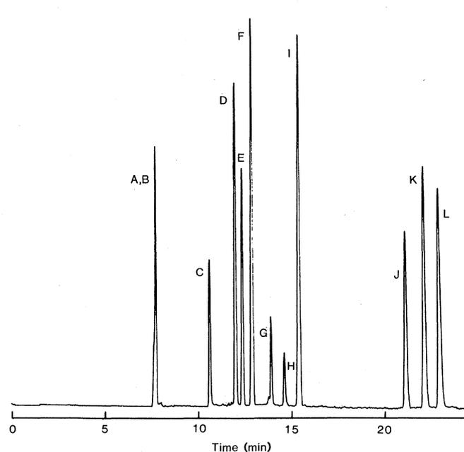
Fig. 4 (left). Electropherogram of fluorescamine-labeled human urine. Conditions as in Fig. 2. [From (14)] Fig. 5 (right). Electropherogram of dansyl amino acids (conditions as in Fig. 2): peak A, unknown impurity; peak B,  $\epsilon$ -labeled lysine; peak C, dilabeled lysine; peak D, leucine; peak E, serine; peak F, glycine; peaks G and H, unknown impurities; peak I, dilabeled cystine; peak J, glutamic acid; peak K, aspartic acid; and peak L, cysteic acid. [From (14)]
