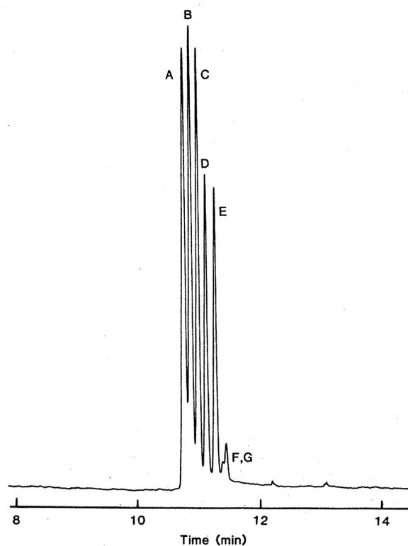
Fig. 3 (right). Electropherogram of *n*-alkylamines as fluorescamine derivatives (conditions as in Fig. 2): peak A, octyl; peak B, heptyl; peak C, hexyl; peak D, pentyl; peak E, butyl; peak F, unknown impurity; and peak G, propyl. [From (15)]
