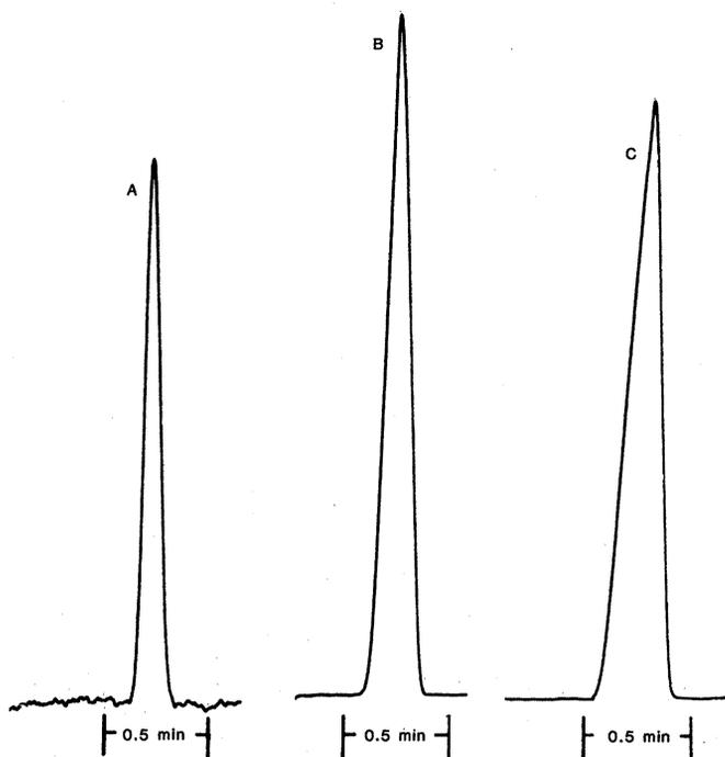
Fig. 2 (left). Effect of sample concentration on zone profile. Glass capillary, 75  $\mu\text{m}$  (inner diameter) by 100 cm long, filled with 0.05M phosphate buffer at pH 7; potential, 30 kV. Dansyl leucine at peak A, 0.4 mM; peak B, 5 mM; and peak C, 10 mM. [From (14)]
