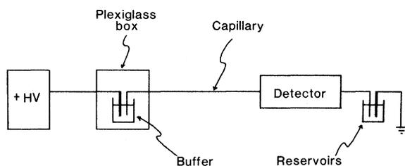
Fig. 1. Schematic of a capillary electrophoresis system.
