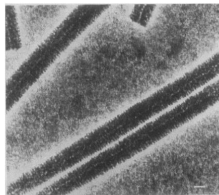
Fig. 9 (right). STEM micrograph of tobacco mosaic virus. The image was obtained with the annular detector and therefore represents elastically scattered electrons. The virus was stained with 1 percent uranyl acetate. Some structure from the scan system can be seen in the image. This can be removed optically if necessary (see Fig. 7). Scale bar, 100 Å; electron dose, 11 electrons per square angstrom. [Micrograph by M. Ohtsuki]
