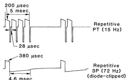
rate of change of the magnetic field ( $dB/dt$ ) was approximately 0.1 G/ $\mu$ sec for PT's and 0.05 G/ $\mu$ sec for SP's (15). Frequency content of the two pulses, derived by discrete Fourier transforms, differs significantly (16).
