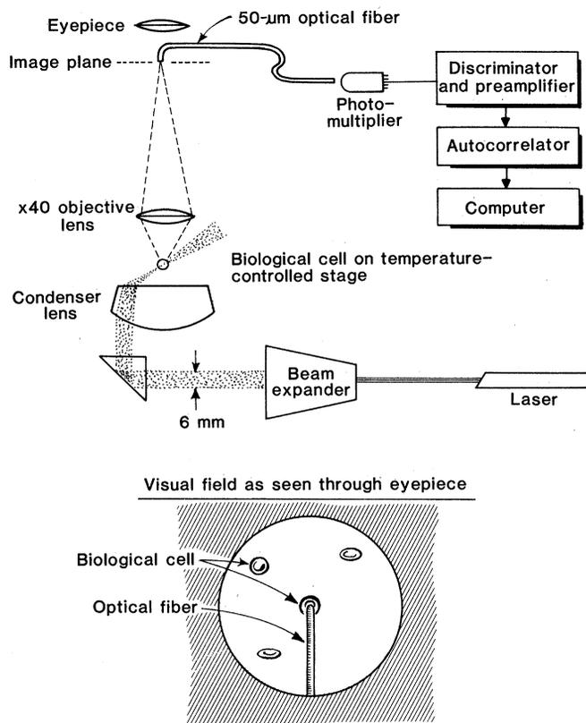
Fig. 1. Schematic diagram of the laser light scattering apparatus used to study the Brownian motion of a local region of cytoplasm in a single red blood cell. An optical fiber embedded in the eyepiece of the microscope collects only light scattered from a volume of  $2\ \mu\text{m}^3$ , allowing characterization of the extent of hemoglobin aggregation in the cell.
