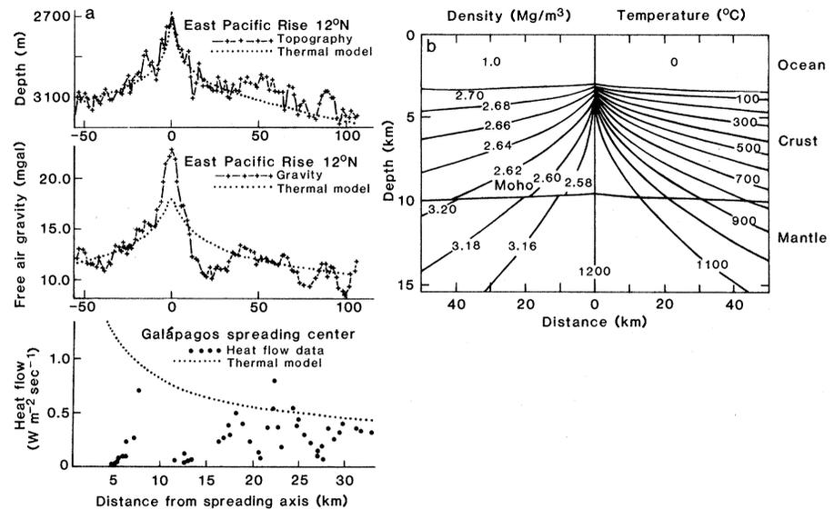
Fig. 4. (a) Bathymetry and gravity data from 12°N and heat flow data from the Galápagos spreading center compared to predictions from the thermal model with a conductively cooled crust. The gravity data are higher and the heat flow data lower than the model predictions. (b) Densities and temperatures from the thermal model with a conductively cooled crust. The topography, gravity, and heat flow data from this model are shown in (a).
