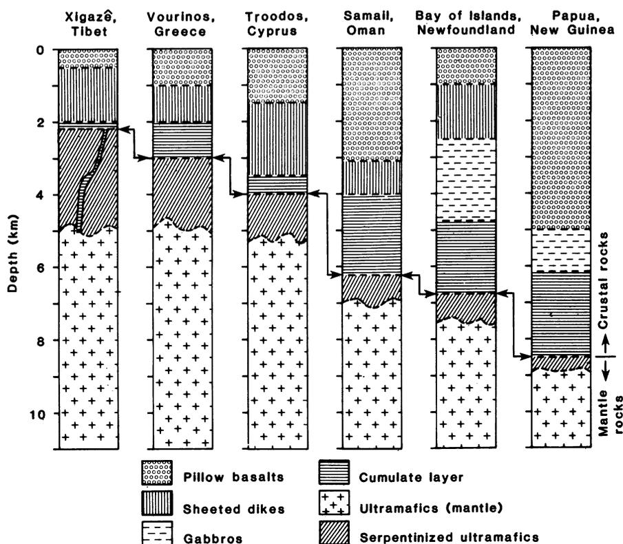
Fig. 1. Schematic sections of ophiolites (5, 6). The basaltic section varies in thickness from 2 km (Xigazê) to about 8.5 km (Papua).
