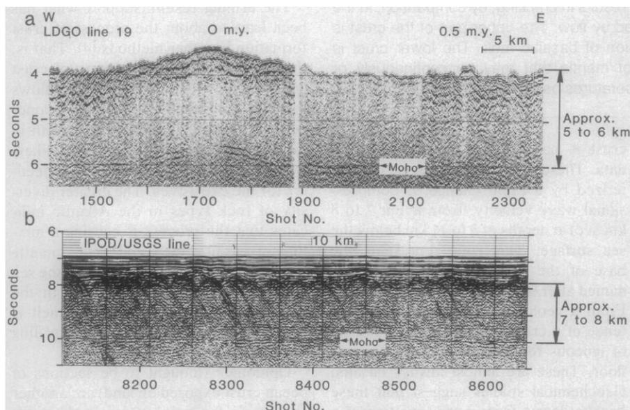
Fig. 2. Multichannel seismic reflection profiles from (a) the East Pacific Rise at 9°30'N (8) and (b) Atlantic crust 135 million years (m.y.) old. The seismic Moho occurs at a two-way travel time of about 2.1 seconds in both profiles. There is no evidence of an increase in travel time under the East Pacific Rise axis due to low-velocity magma.
