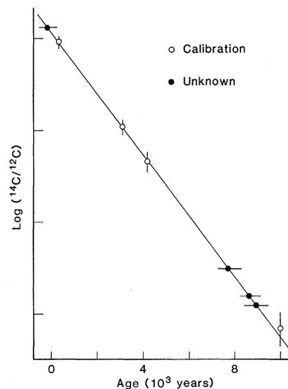
Fig. 2. Results: (○) calibration points fit with a half-life of 5568 years; (●) data from samples of unknown age.
