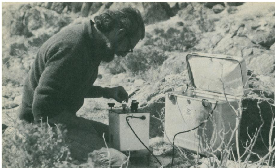
Measuring relative elevation changes with a gravimeter
