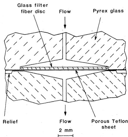
Fig. 3. Enlarged diagram of reaction cartridge for gas phase sequenator (10). [Courtesy of the *Journal of Biological Chemistry*]
