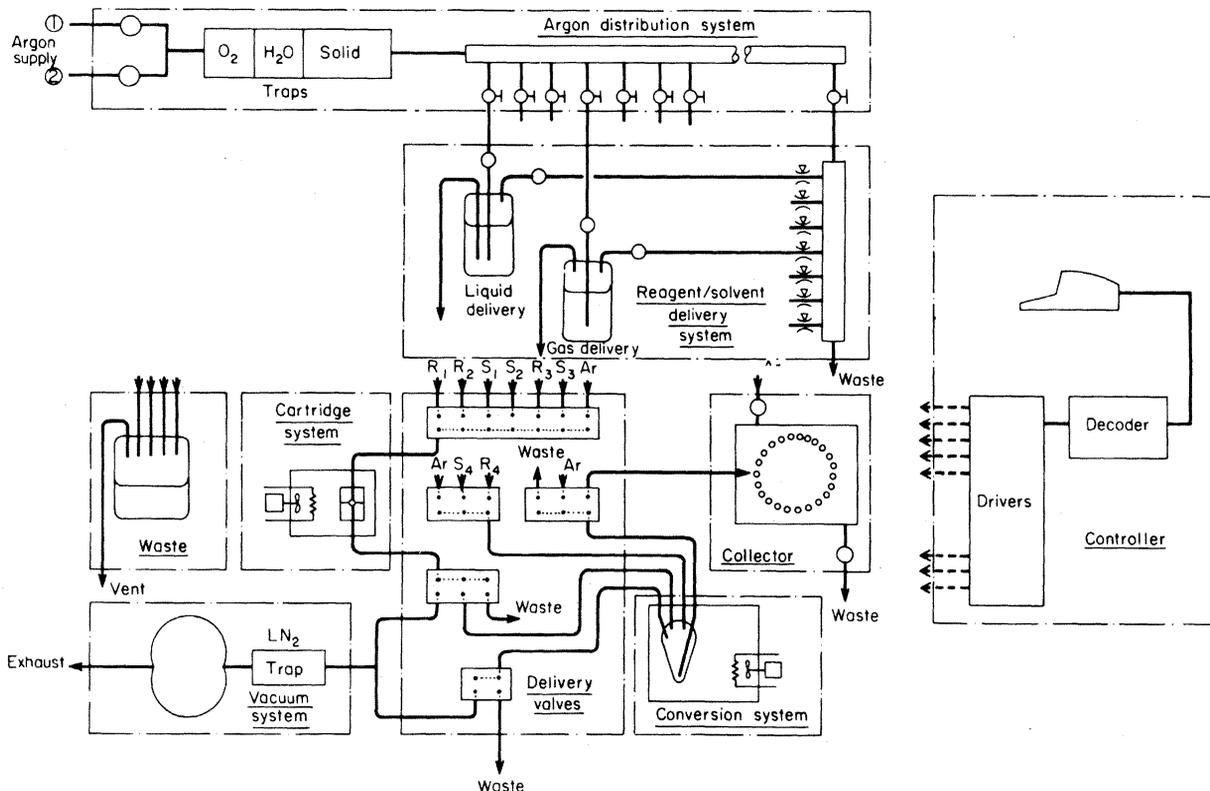
Fig. 2. Schematic diagram of gas phase sequencer (10). [Courtesy of the *Journal of Biological Chemistry*]
