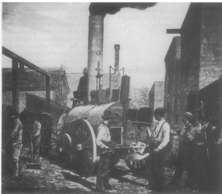
"This traveling garbage burner meandered through the alleys of Chicago in 1893. It operated at a total cost of about twenty dollars a day." [Reproduced from Scientific American in Garbage in the Cities ]
