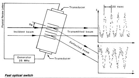
A light beam passing through the switch changes direction every 10 nanoseconds.
