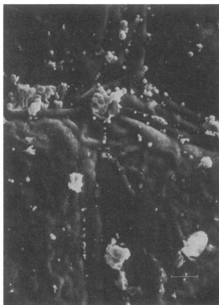
Fig. 1. Adaxial surface of a chestnut oak leaf ( Quercus prinus ) collected in the upper canopy (scale bar, 30 \mu m). Deposited particles (resolution, ~ 0.5 \mu m) are heterogeneously distributed on the leaf, often occurring as aggregates in surface irregularities of the leaf.
