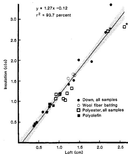
Fig. 1. Thermal insulation of various clothing materials, plotted against swatch loft as measured on the heat transfer apparatus. The shaded area delineates the 95 percent confidence limits and the asterisks indicate swatches that had multiple layers.
