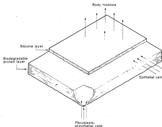
Fig. 1. Schematic representation of a standard version of the noncellular bilayer polymeric membrane (stage 1). The moisture flux through the layers ranges from 1 to 10 mg/cm<sup>2</sup> per hour. Fibroblasts and endothelial cells migrate into the bottom layer while epithelial cell sheets advance from the wound edge in the plane of the membrane, between the two layers. The top layer is a conventional medical-grade silicone which undergoes cross-linking at
