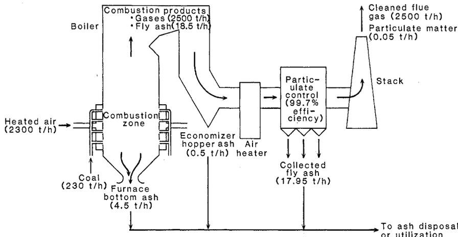
Fig. 1. Schematic of a 500-MW, coal-fired power plant, illustrating the origin and major paths of the fly ash, assuming a typical coal with a 10 percent ash content. Of the 23 tons per hour (t/h) of ash introduced into the boiler with the coal, all but 0.2 percent is collected for subsequent disposal or use. Advanced particulate emission control technologies will reduce this emission to less than 0.1 percent.
