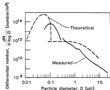
Fig. 5. Comparison of theoretical particle number distribution and distribution based on field measurements. The theoretical prediction (31) is based on input parameters from the boiler. Qualitative agreement in the region of the submicrometer mode is considered good. The theory is based on a model of particle formation involving volatilization and condensation of fly ash during coal combustion.
