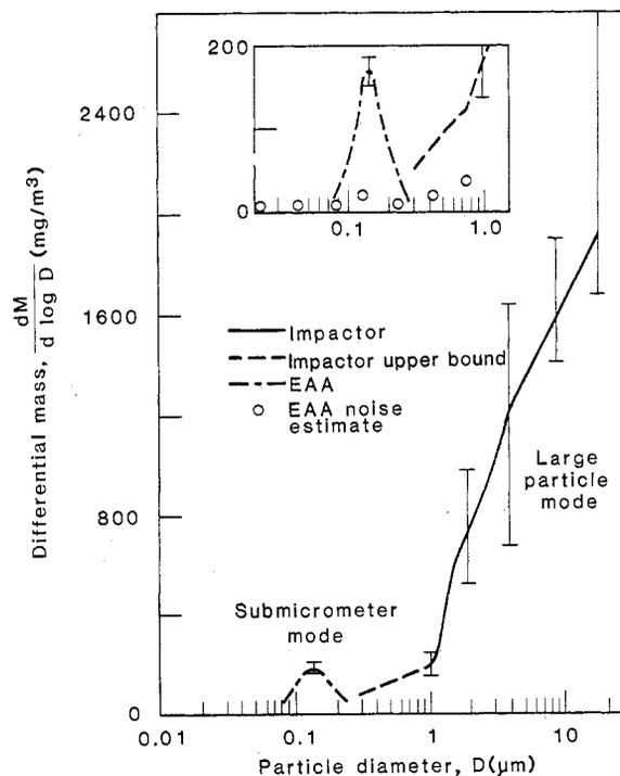
25). Flue gas samples were diluted, typically by a factor of 80, to reduce the aerosol concentration to within EAA limits, and the charge on the particles was neutralized with radioactive sources before introduction to the EAA (26, 27). The EAA was the primary instrument used to measure size distributions of particles below 0.5  $\mu\text{m}$  in diameter.
