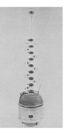
for each application. System comprises eight bubble cap sections, eight sampling units, a liquid divider, a coaxial condenser, a boiling flask, product receiver, heating mantle, framework, and clamps. Systems are available in several diameters. Kontes. Circle 837.
