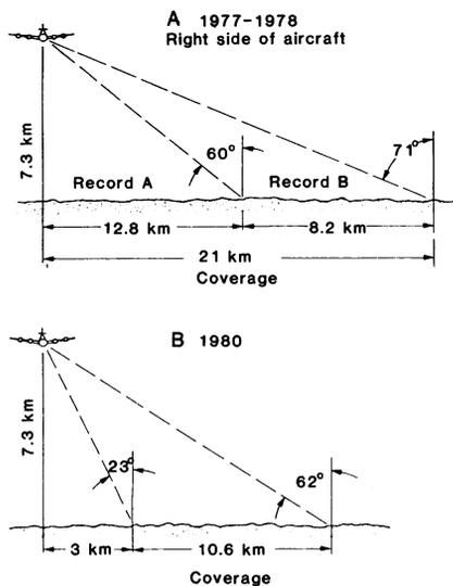
Fig. 2. Radar acquisition geometry.
