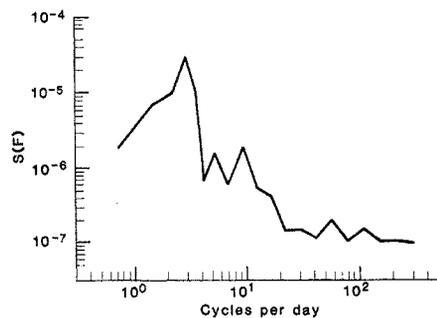
Fig. 3. A 34-hour measurement of the spectrum of the background noise of the dual-channel microwave radiometric system; the ordinate is lower by a factor of  $10^3$  than in Fig. 2. The units of the ordinate are square centimeters per cycle per day.
