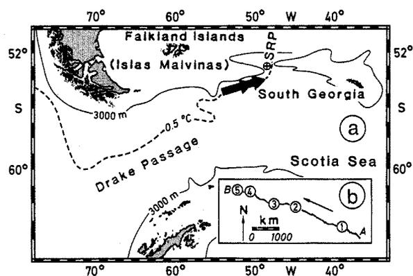
Fig. 1. (a) Position of the near-bottom, long-term current meter mooring in the Shag Rocks Passage (SRP), Scotia Sea; (b) the progressive vector diagram of the 2973-m instrument, 35 m above the sea floor. The 3000-m isobath and 0.5°C isotherm have been adapted from Gordon (6), who has predicted strong bottom currents (double arrow) west of the SRP. The numbers in (b) denote periods of overflow as seen in Fig. 2c.
