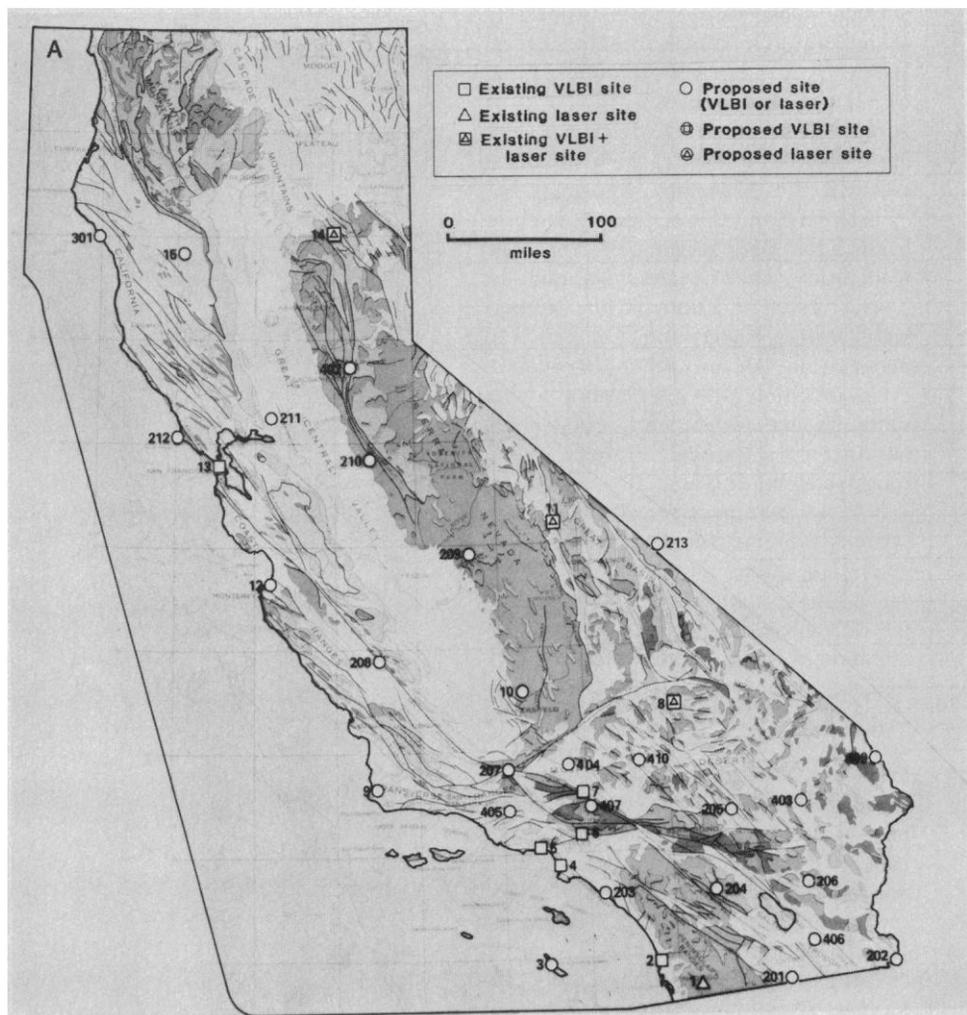
Fig. 3. (A) VLBI observatories and sites planned for mobile VLBI and laser station occupation in California. (B) Observatories and mobile station sites in North America (24). Notation used in the figure is explained in (24).
