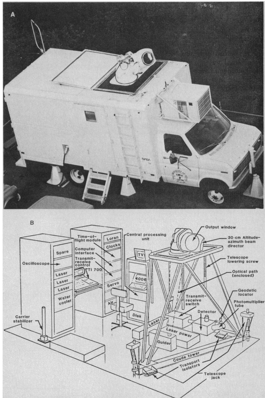
Fig. 1. (A) Transportable laser ranging station, with telescope beam director deployed for ranging. (B) Block diagram of the TLRS interior. [Photograph courtesy of McDonald Observatory, University of Texas, Austin]
